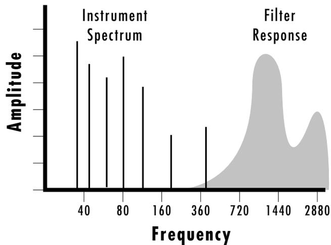
*The Filter can only act on frequencies that are present in the Instrument. Use the Filter Frequency Tracking control to “fine tune” the filter to the instrument. No sound would be output from the example above because the filter's frequency response and the harmonic spectrum of the instrument do not coincide.*
