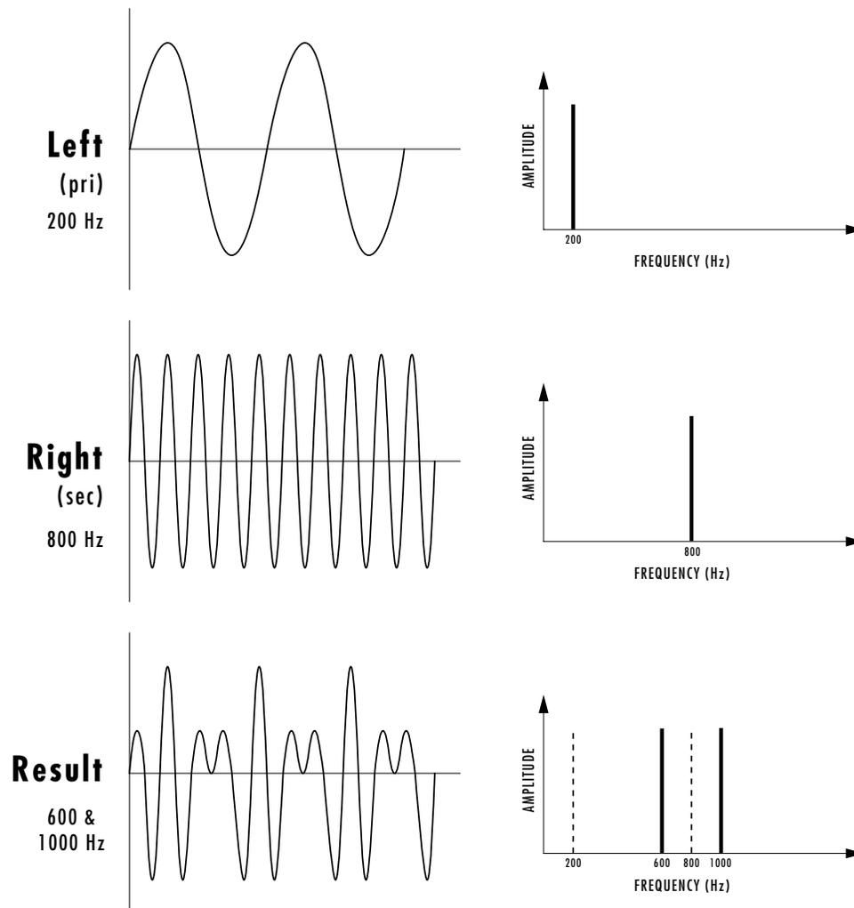
*This diagram shows the result of Ring Modulating two sine waves with frequencies of 200 Hz and 800 Hz. Only the Sum and Difference frequencies of 1000 Hz and 600 Hz will result.*
