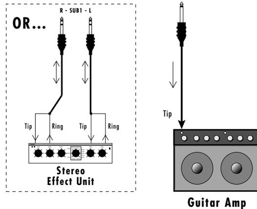
*Using the programmable outputs and returns, specific presets can be routed through outboard processors without using up precious mixer channels.*
