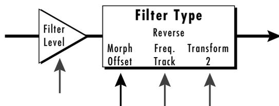
The filter has an input level control called the *Filter Level* which controls how much signal is presented to the filter. This control (like most of the controls in UltraProteus) has an initial amount and can also be controlled from a note-on modulation source. Certain UltraProteus filters are designed to distort the signal as a musical effect. The Filter Level allows you to control the amount of distortion produced by these special filter types.
