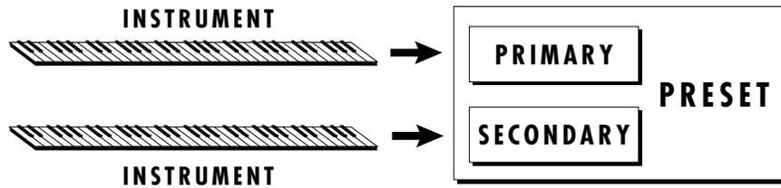
The primary and secondary layers of the preset are essentially two instruments with complete modulation controls. The memory is organized into banks of 128 programmable RAM presets, unalterable ROM presets and Hyperpresets.
