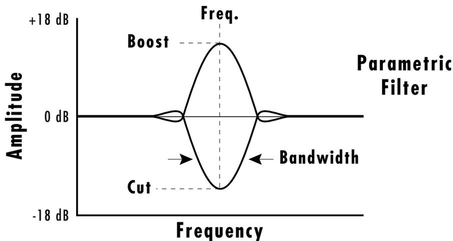
The parametric filter is quite flexible. Any range of frequencies can be either amplified or attenuated. Often times, several parametric sections are cascaded (placed one after another) in order to create complex filter response curves.
