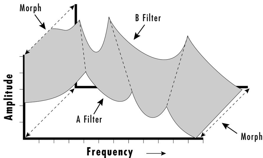
*The UltraProteus Z-plane filter has the unique ability to change its function over time.*
