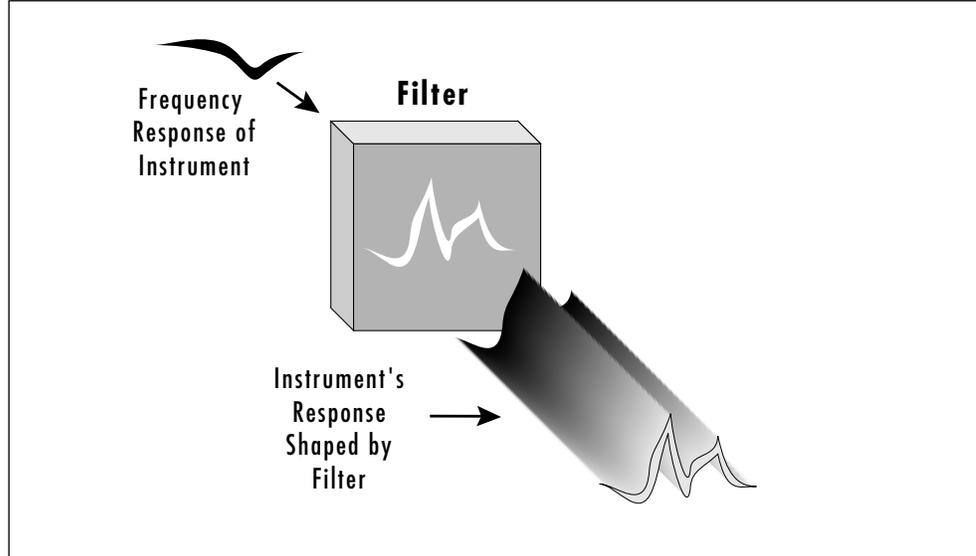
Of course, the filter cannot amplify or attenuate frequencies which do not exist in the original instrument. The Filter Frequency Tracking control can be used to “tune in” the filter to match the instrument.
